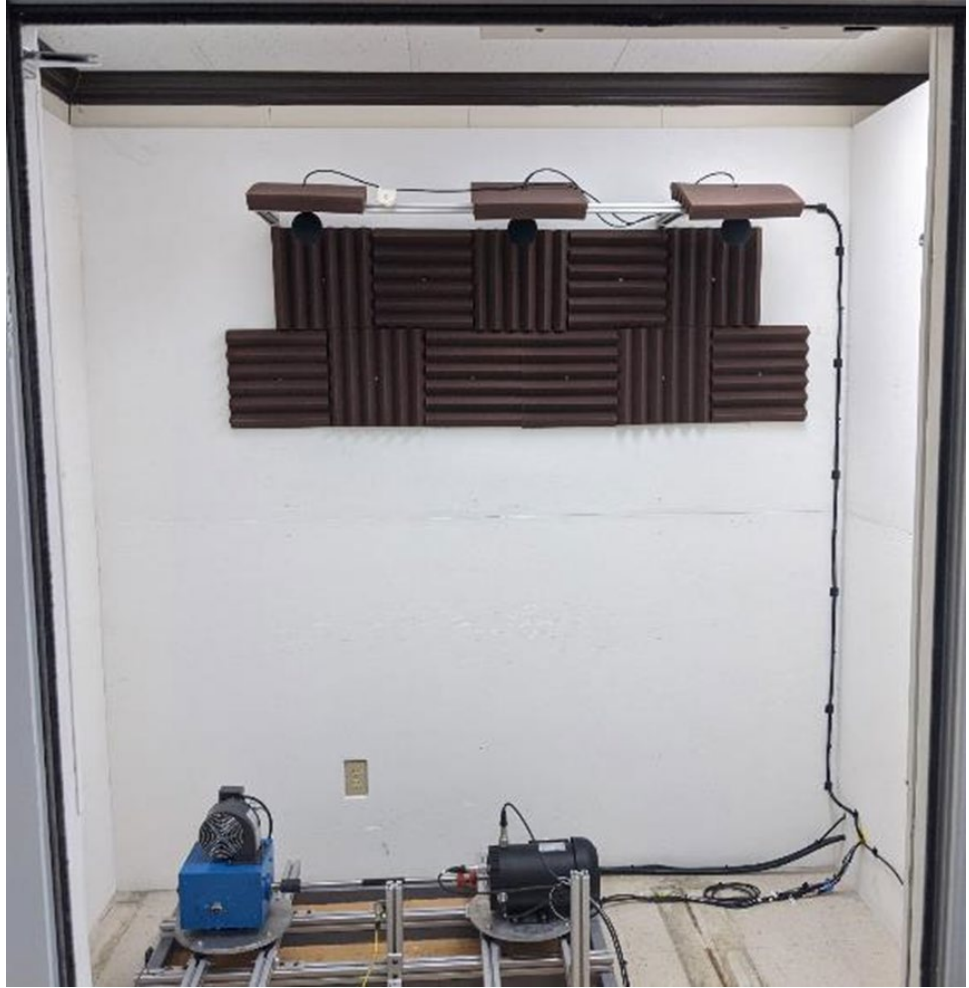
Figure 3-2 Acoustic array installed in the test chamber
