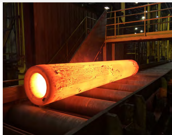
Extruded Pipe Extrusion - Inconel 740H (22" OD x 3.7" W x 14' L)
