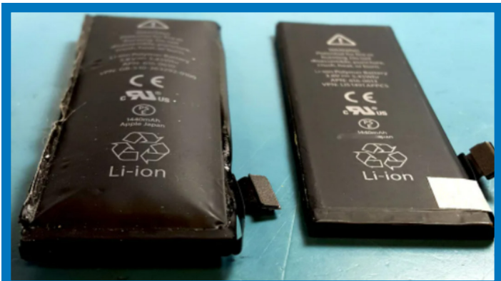
Figure 4 – Side-by-side comparison of a lithium ion polymer pouch cell that has undergone the onset of thermal runaway (left) and an undamaged cell (right) [10]. Image courtesy of Appuals.
