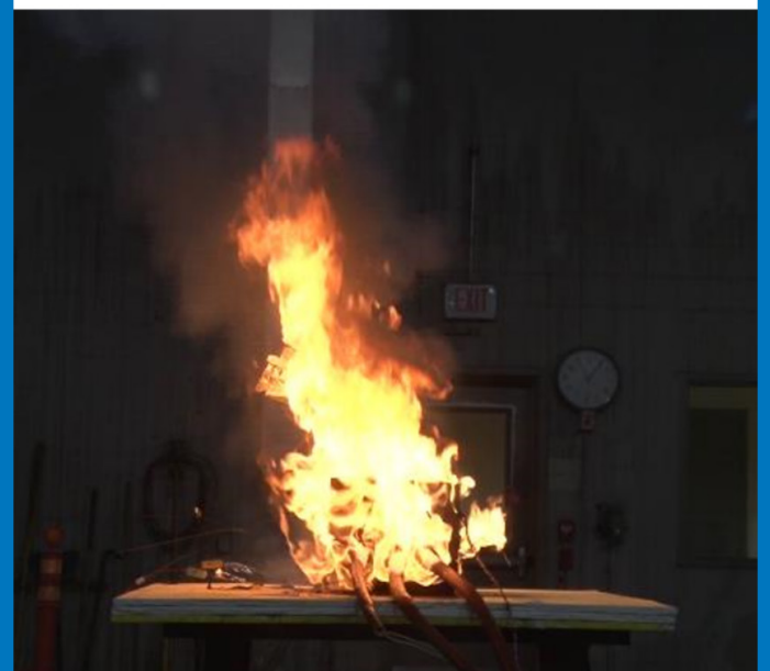
Figure 5 – Lithium ion battery module thermal runaway leading to flammable gas release (left) and fire (right). Images courtesy of FM Global. Testing involved overheating of lithium iron phosphate cells without the presence of an external ignition [9].
