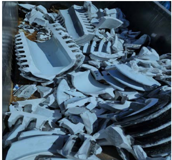
Figure 5. Illustration of Destroyed OIP Bushing Sheds
