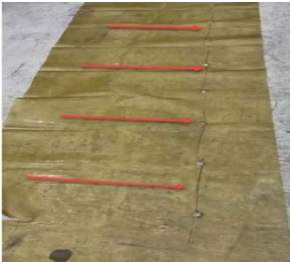
Figure 16. Punctured Insulation Because of Leakage Path Overcomes the Dielectric Strength
