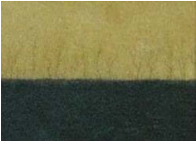
Figure 19. Image of Bushing Failure "Trees Trace" with Signs of Copper Sulfide Migration
