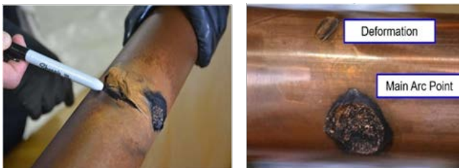
Figure 11. Illustration of the Main Arc Point and Deformed Center Conductor
