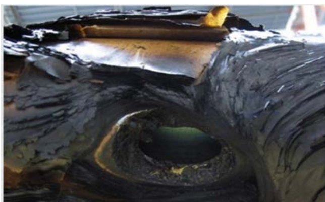
Figure 13. Illustration of 345-kV Bushing: Close-Up of the Major Fault Location Through the Insulation to the Center Conductor
