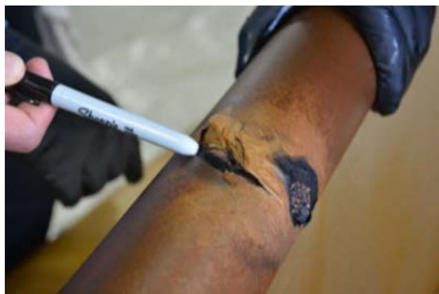
Figure 7. B-Phase Extended Internal Damage of 230-kV Bushing with Copper Center Conductor
