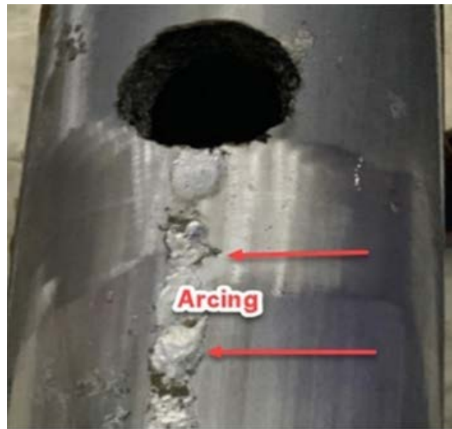
Figure 17. Illustration of Punctured Conductor with Signs of Arcing and Burning
