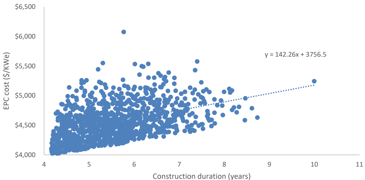
Figure 3-2. Construction duration versus EPC cost (conventional LWR)
