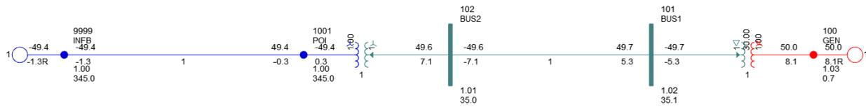
Figure 3. Example aggregated IBR plant model.
