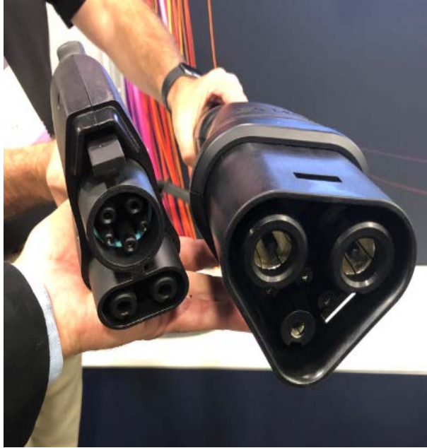
Figure 4. MCS charging connector (right) compared to a CCS charging connector (left)
