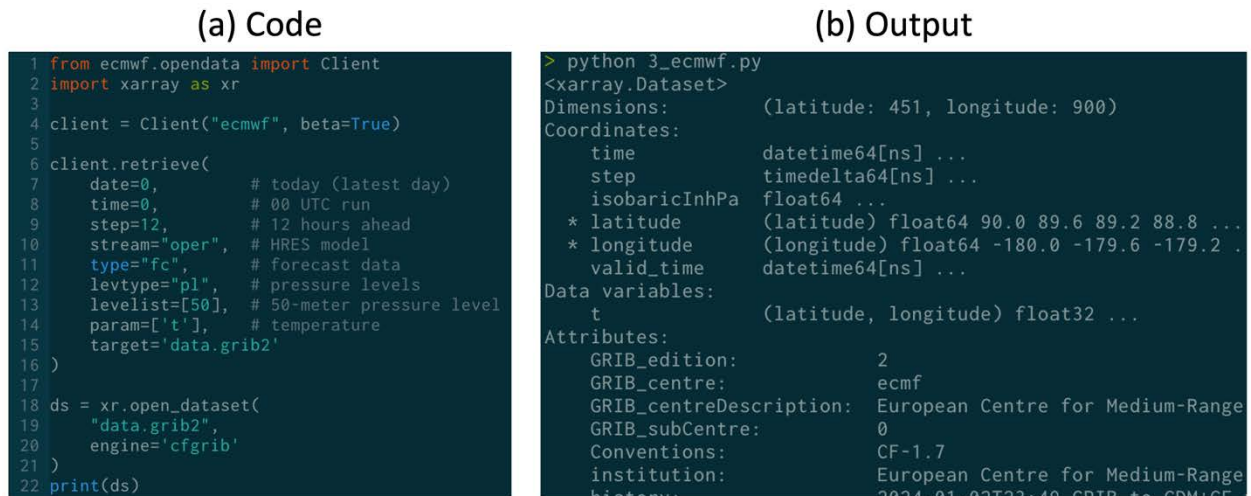
Figure 9. Example of downloading NWP data in Python using the ecmwf-opendata package. The output is clipped for readability purposes.
