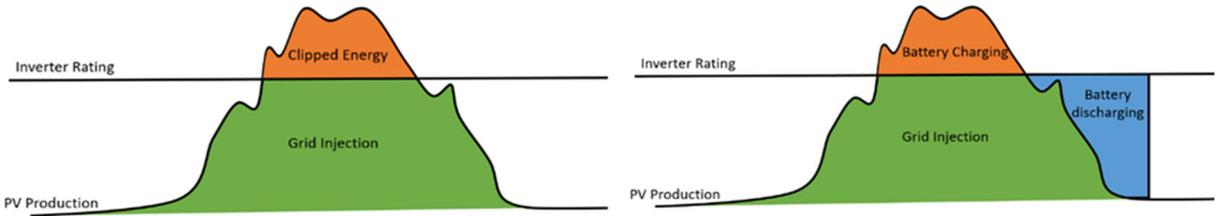
Figure 9. DC-coupled systems have the capability of reducing clipped energy
