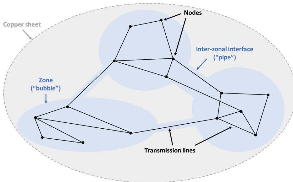
Figure 8. Illustration of transmission system topology modeling options
