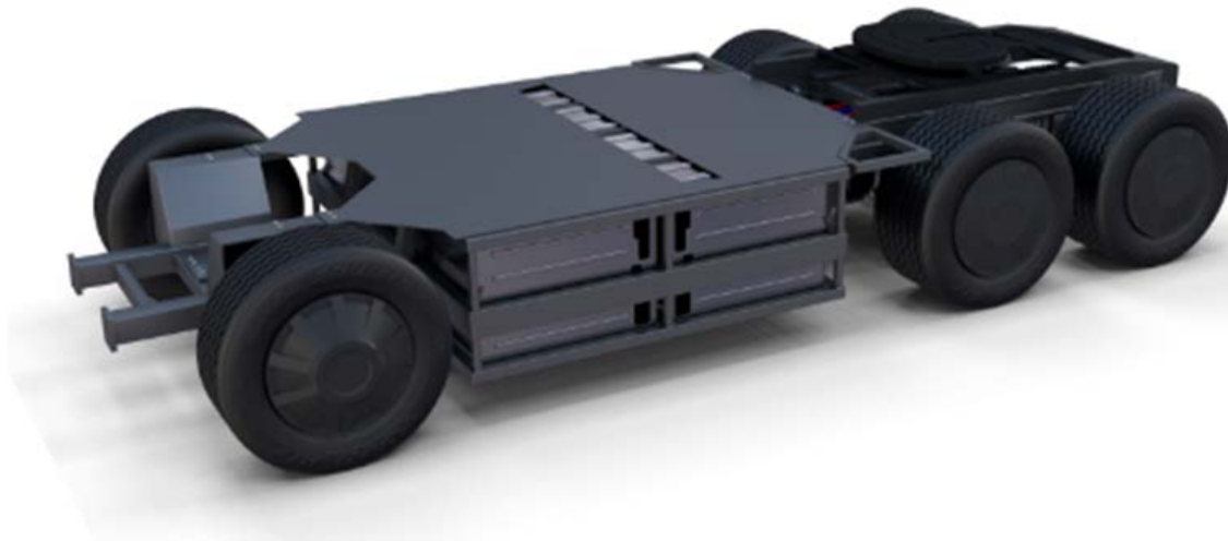
Figure 6. Battery Packs Mounted in Semi-Tractor Chassis
