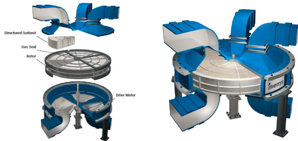
Figure 2-4 Schematic and cutaway of Svante Solid-sorbent rotating bed process. Image courtesy of Svante
