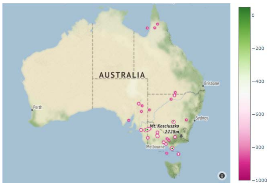
Figure 9. Available MVA at different generator buses displayed on an approximate geographical location. A darker pink shade indicates more negative available MVA and hence greater risk of instability
