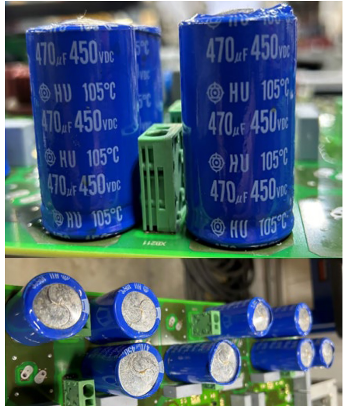
Figure 8. Vented electrolytic capacitor, side and top views
