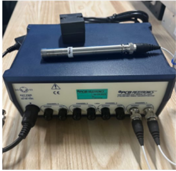
High frequency and low frequency acoustics sensors with signal conditioning box
