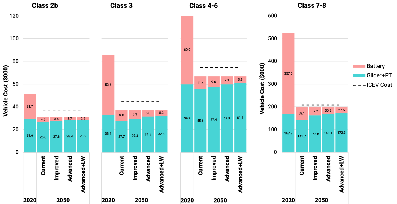
Figure A-2. Medium- and Heavy-Duty BEV Cost Assumptions in US-REGEN. Figure shows projected cost in real $2022 for a representative vehicle in each class, with battery pack costs broken out from other costs, including the glider and non-battery components of the powertrain (PT). Battery pack costs are based on an assumed 150-mile range for Class 2b, 200 miles for Class 3-6, and 500 miles for Class 7-8, reflecting long-haul freight trucks (see Table A1). Total cost of a comparable ICEV is shown for comparison.
