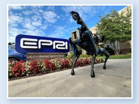
One of EPRI's two Boston Dynamics SPOT units, which have already been used for electrical panel manipulation testing, cybersecruity, and EMI/RFI testing.
