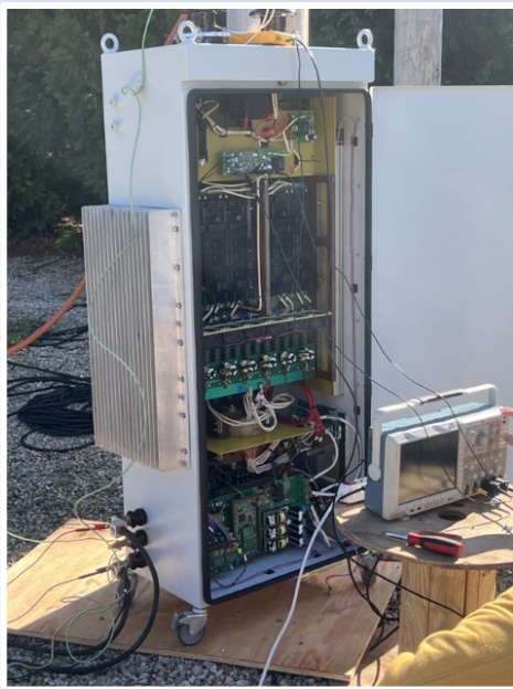
Prototype 25-kVA solid state transformer
