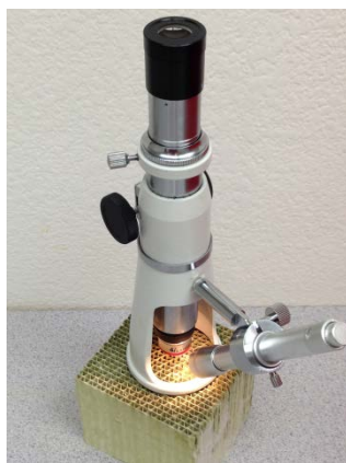
Figure 3-5 Example of Microscope Used to Document Catalyst Cell Dimensions
