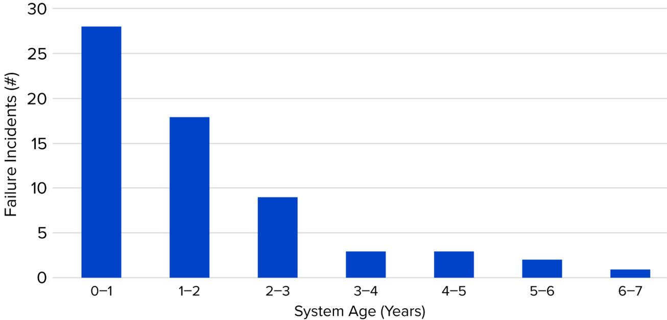
Figure 5. BESS Age at Failure, where known
