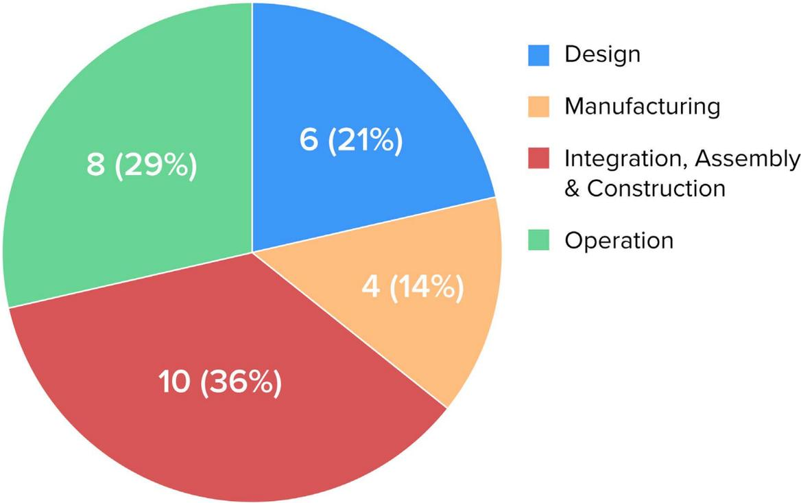
Figure 4. Breakdown of BESS Failures by Root Cause
