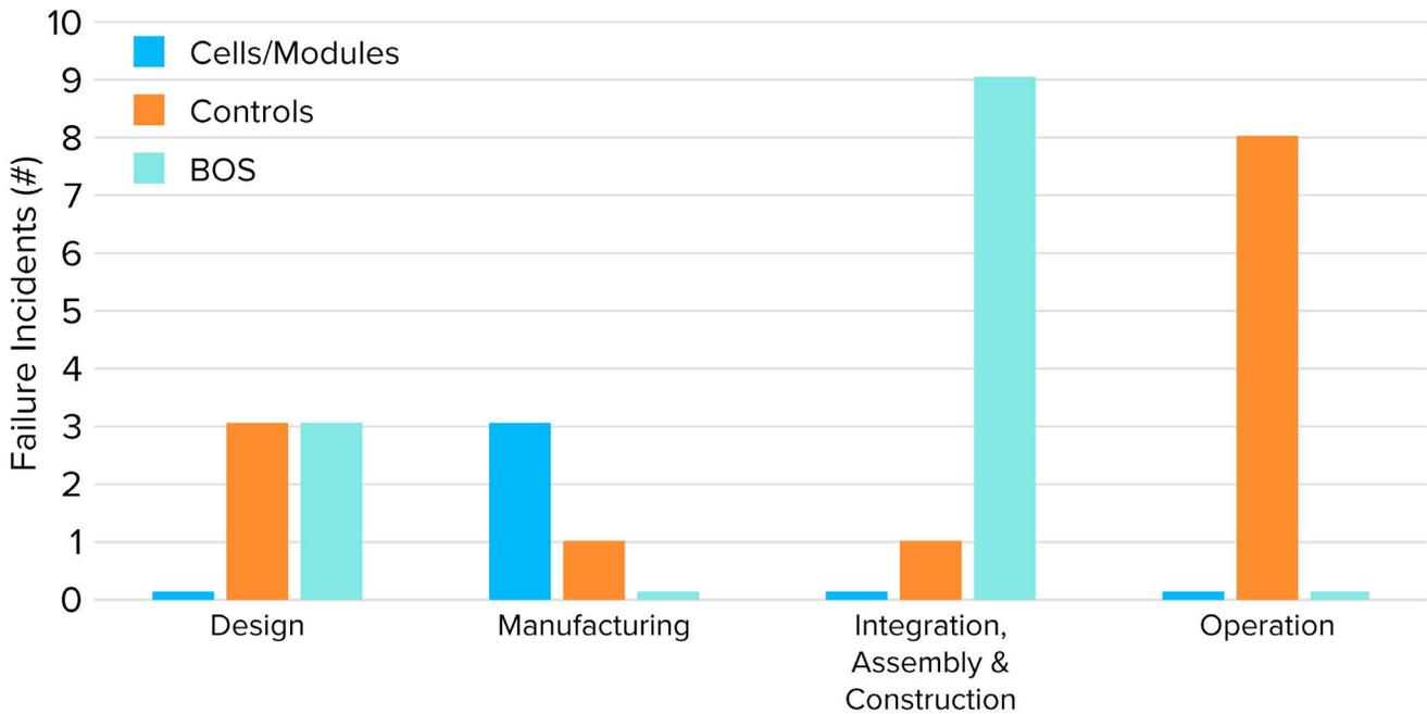
Figure 7. Relationship between Root Cause and Failed Element
