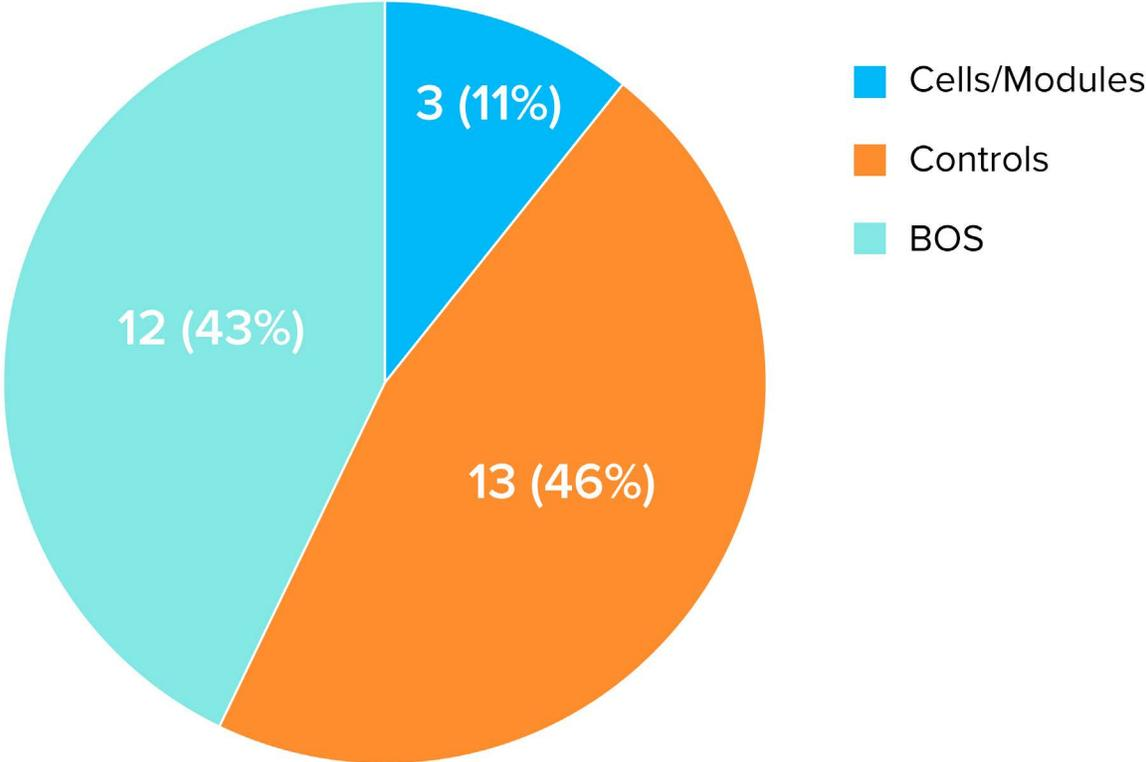
**Figure 6.** Breakdown of BESS Failures by Failed Element
