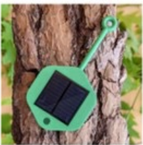
Sensor Solar-powered gas sensors detect wildfires even during the smoldering phase
