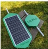
Gateways Distributed LoRa Gateways provide a large-scale mesh network infrastructure
