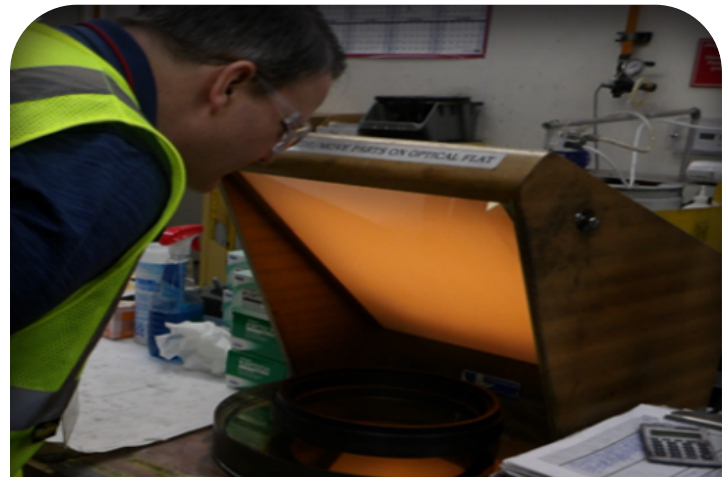
Figure 1. Optical comparator flat with monochromatic light
