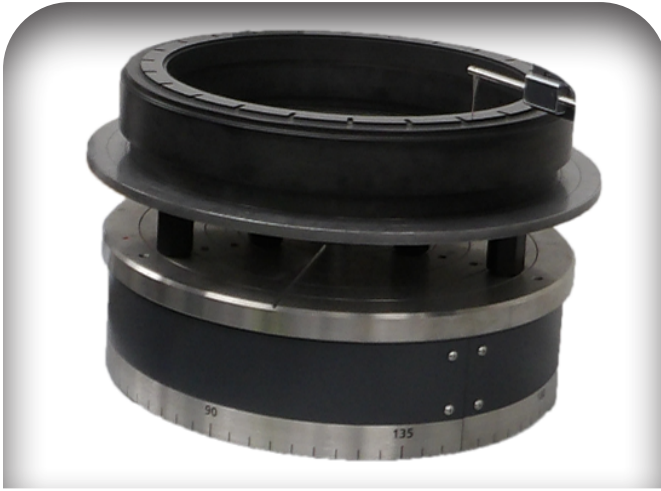
Flatness testing with no holder
