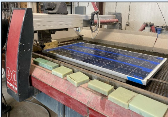
Waterjet cutting of a PV module for toxicity characteristic leaching procedure testing
