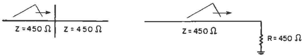
Figure 7-1. Single-phase Surge Impedance Termination
