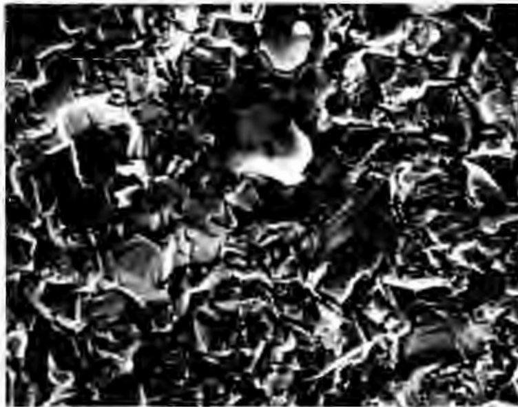
Figure 3-1. SEM Image (1000X)* of Tube R5C40 Surface After Bromine-Methanol Descaling (2.21 EFPY)
