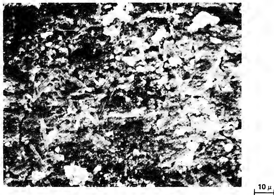
Figure 3-12. SEM Image of Crud From Tube R36C37 at 1000X*(7.02 EFPY)
