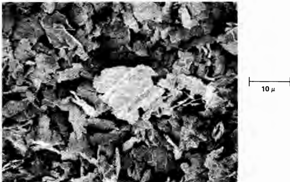
Figure 3-15. SEM Image (1000X)* of Crud Removed From Tube R5C40 Using Electrolytic Descaling Technique (2.21 EFPY)
