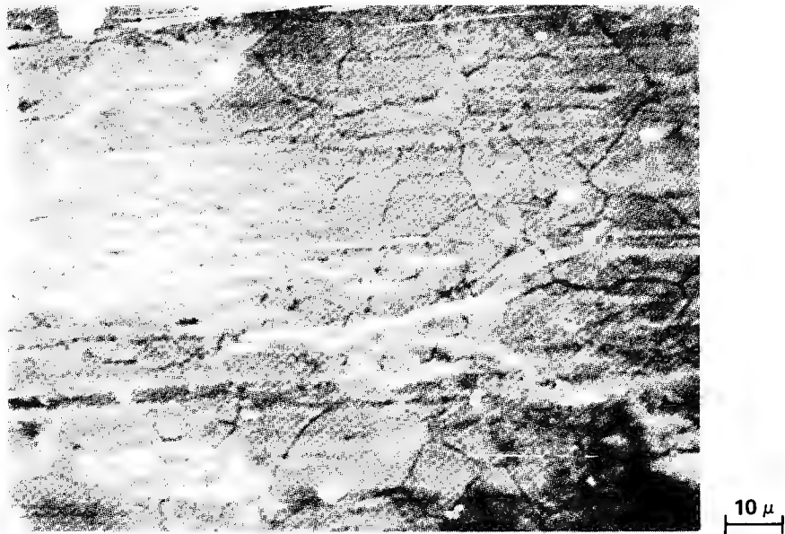
Figure 3-11. SEM Image of Crud From Tube R1C25 at 1000X*(1.75 EFPY)
