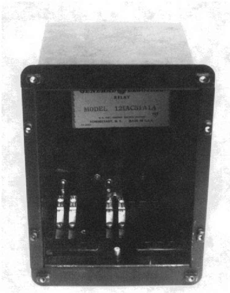
Figure 3-12 Relay Case With Contact Fingers Visible
