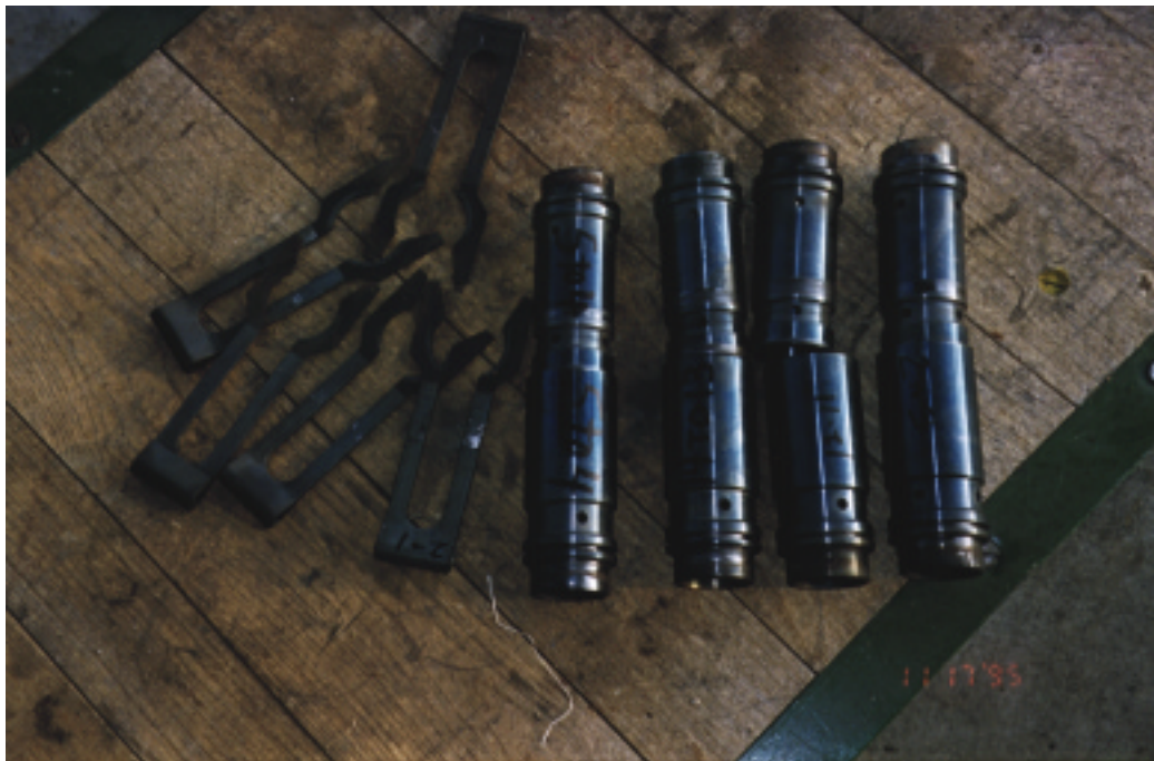
Cross fire tubes typical condition after 4,000-10,000 hours. These fire tubes had 9,682 hours of operation. Figure 8.50 Unit 4B 11/95, 14,264 hrs. Cross Fire Tubes.
