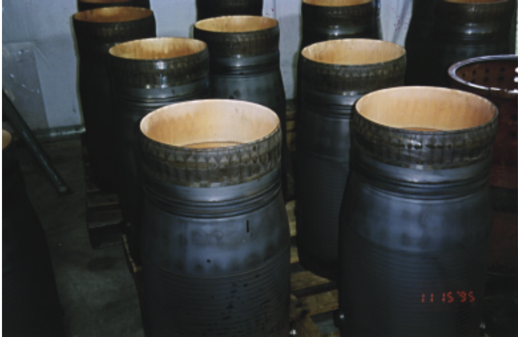
After 9,682 hours of operation the combustor liner appears in good condition. Figure 8.44 Unit 4B 11/95, 14,264 hrs. Combustion Liner.
