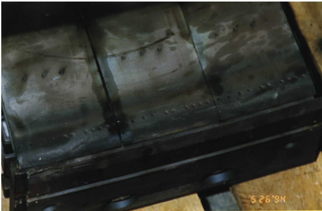
1st stage stationary shroud. good condition with no rubs. Figure 8.32 Unit 3B 5/94, 4,082 hrs. 1st Stage Stationary Shroud.
