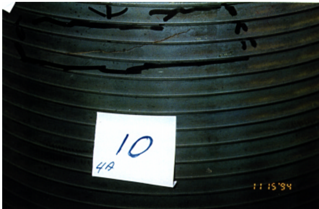
Figure 12 Unit 4B 11/95, 14,264 hrs. Combustion Liner.
