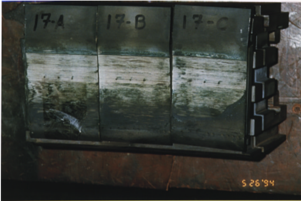
1st stage stationary shroud horizontal flange shows a substantial rub. Figure 8.33 Unit 3B 5/94, 4,082 hrs. 1st Stage Stationary Shroud.
