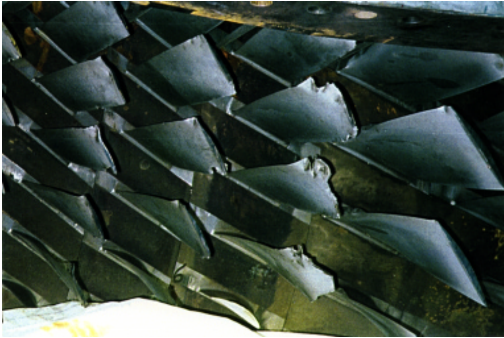
Compressor rotor section blade failures. Figure 5 Unit 4A 2/95, 6,120 Hrs. Compressor Rotor
