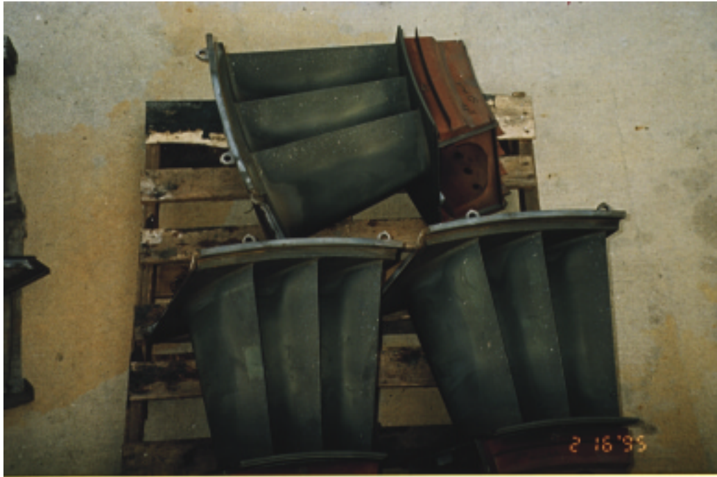
3rd stage nozzle showing minor damage from compressor blade impactions. Figure 8.31 Unit 4A 2/95, 6,120 hrs. 3rd Stage Nozzle.
