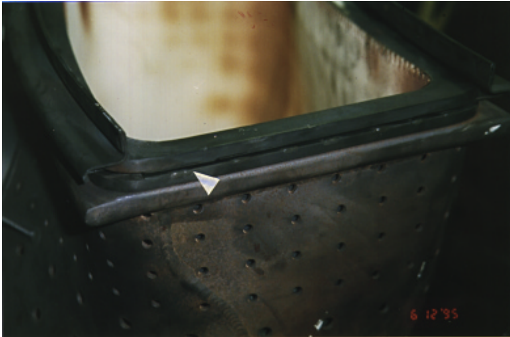
Transition piece showing design modification resulting in minimal wear. Figure 8.55 Unit 3B 6/95, 12,586 hrs. Transition Piece.
