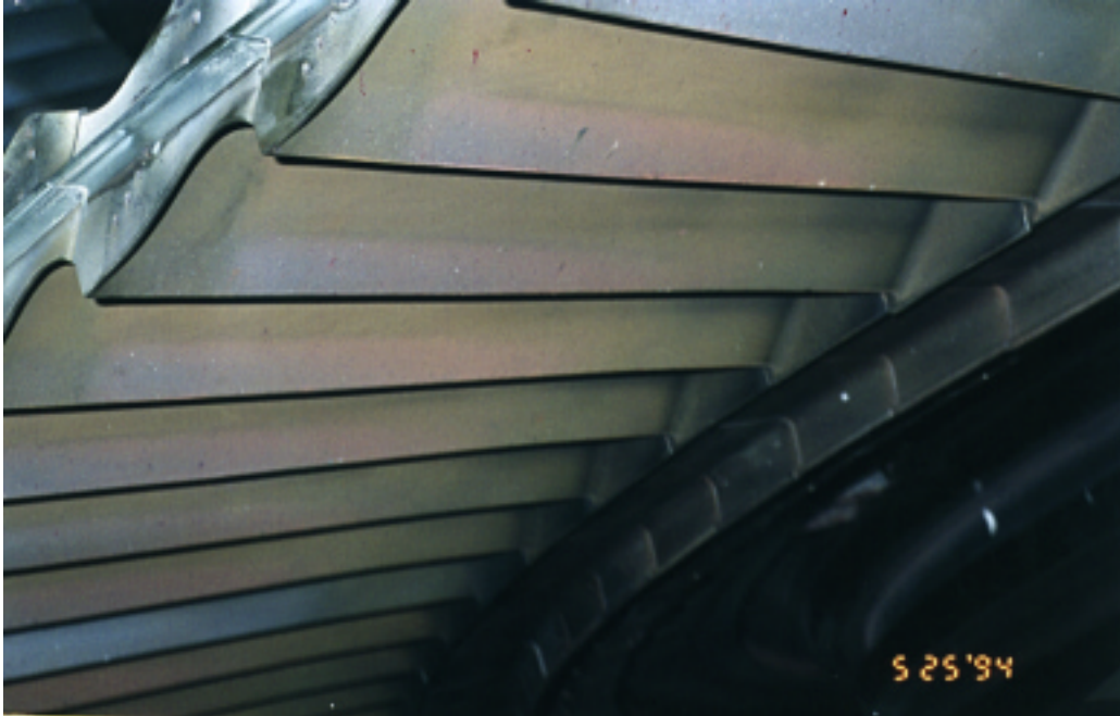
2nd stage buckets viewed from the trailing edge side. Figure 8.13 Unit 3B 5/94, 4,082 hrs. 2nd Stage Buckets.
