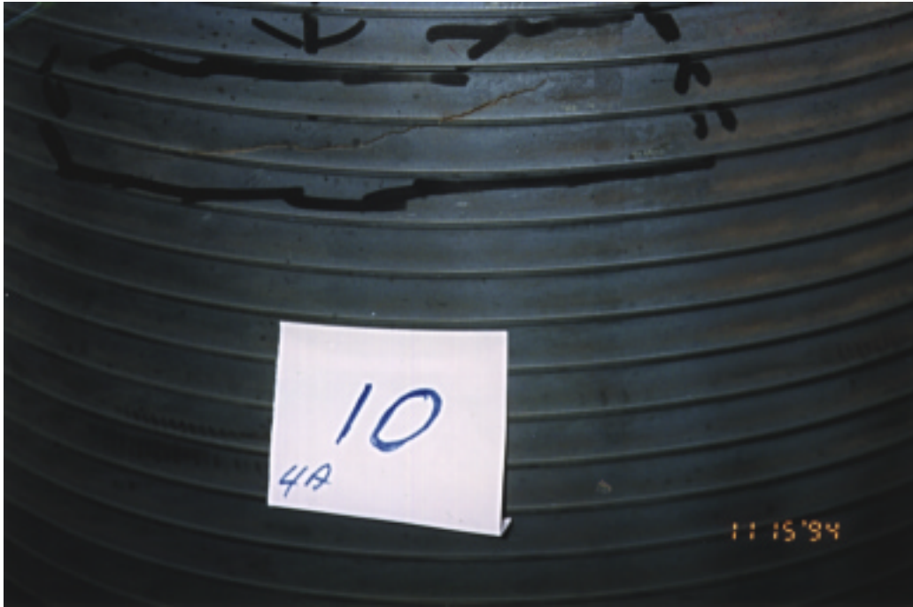
Combustion liner showing body crack, after 4,868 hours. (Seen in one liner only). Figure 8.49 Unit 4A 11/94, 4,868 hrs. Combustion Liner.
