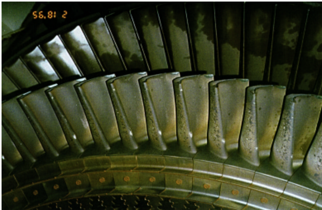
The 1st stage buckets are shown after the impactions from the compressor blades. Figure 6 Unit 4A 2/95, 6,120 hrs. 1st Stage Buckets.
