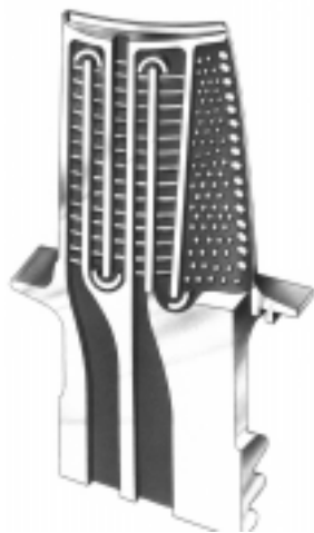
Cooling in the 1st Stage Blade
