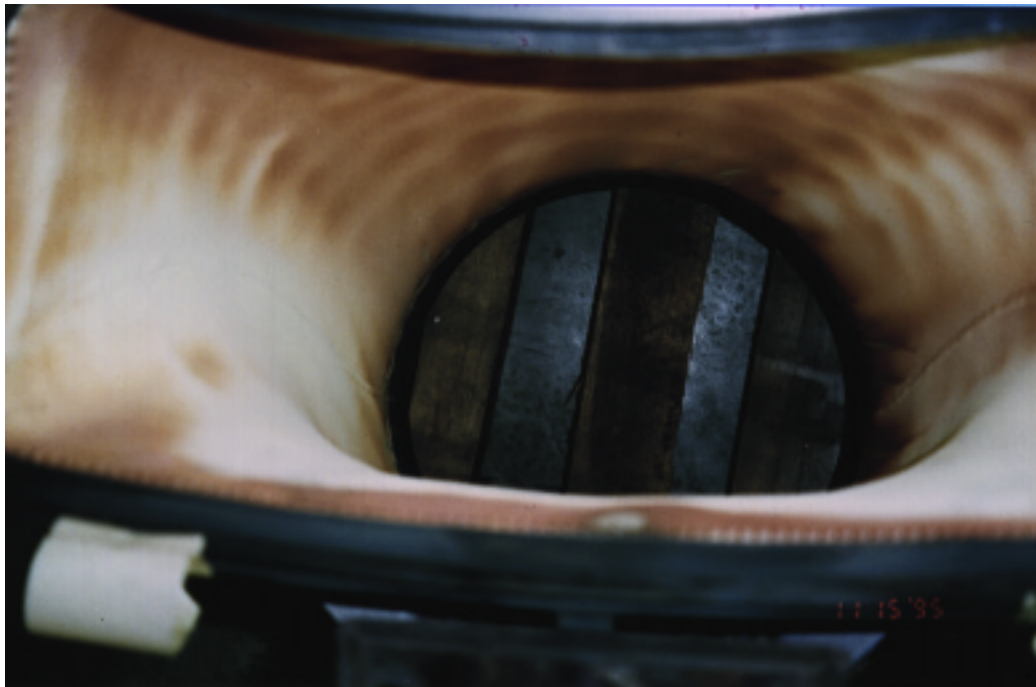
Transition piece in good condition, after 9,682 hours. Figure 8.56 Unit 4B 11/95, 14,264 hrs. Transition Piece.
