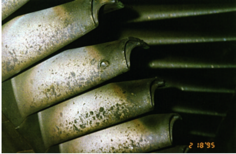
1st stage buckets showing convex side damage from compressor blade impactions. Figure 7 Unit 4A 2/95, 6,120 hrs. 1st Stage Buckets.
