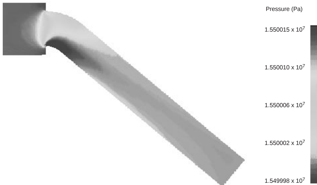
Figure B-3-5 Pressure Field in the Middle Vertical Plan (Contraction Model)
