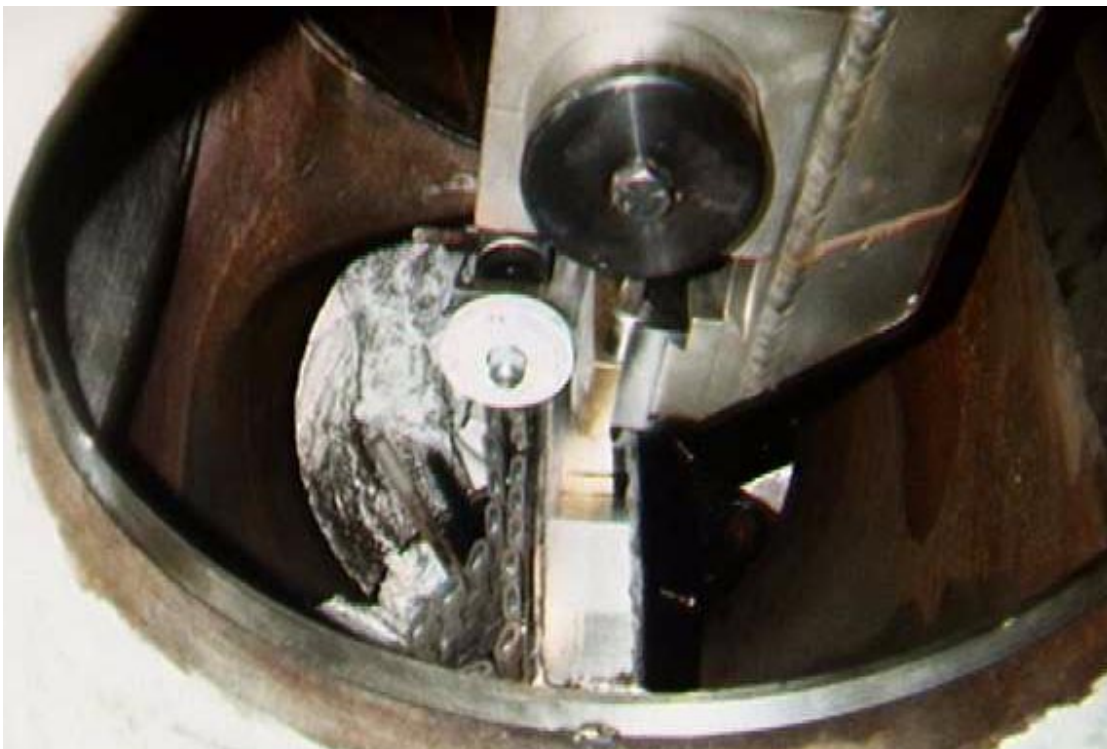
Figure 4-6 RFO8 Machining Mockup - Polishing Wheel
