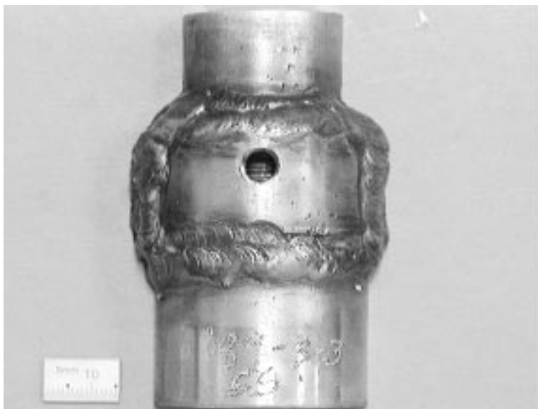
Figure 4-26 Exterior of Stainless Steel Threaded Pipe Cap Coupon Repaired Using Split Collar
