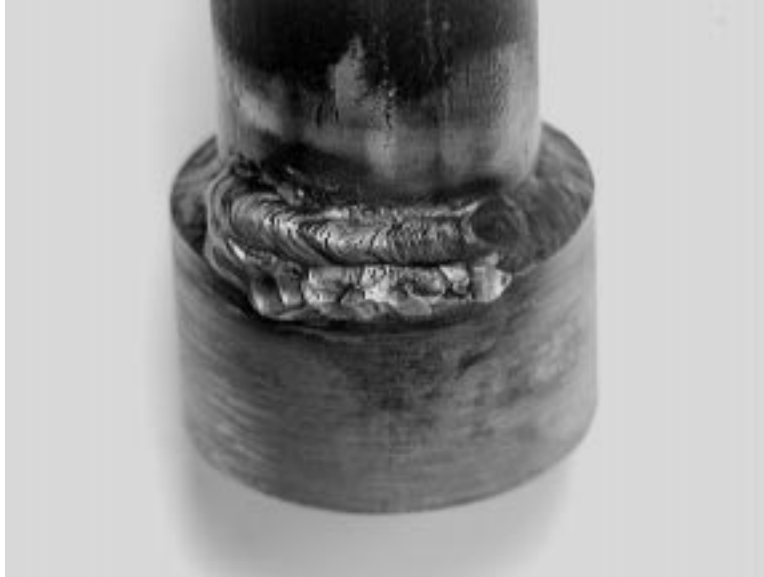
Figure 4-3 Test Coupon CSS-1 after Welding
