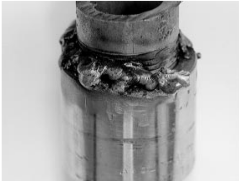
Figure 4-21 Test Coupon SST-2 after Welding
