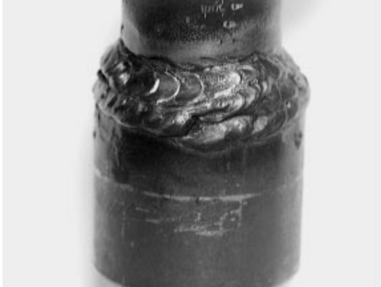
Figure 4-14 Test Coupon CST-5 after Welding
