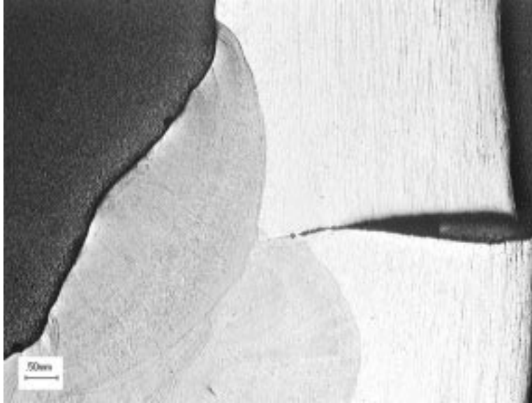
Figure 4-16 Cross-Section of Coupon SSS-1 Showing EDM Notch Sealed by Welding (Magnified 10x)
