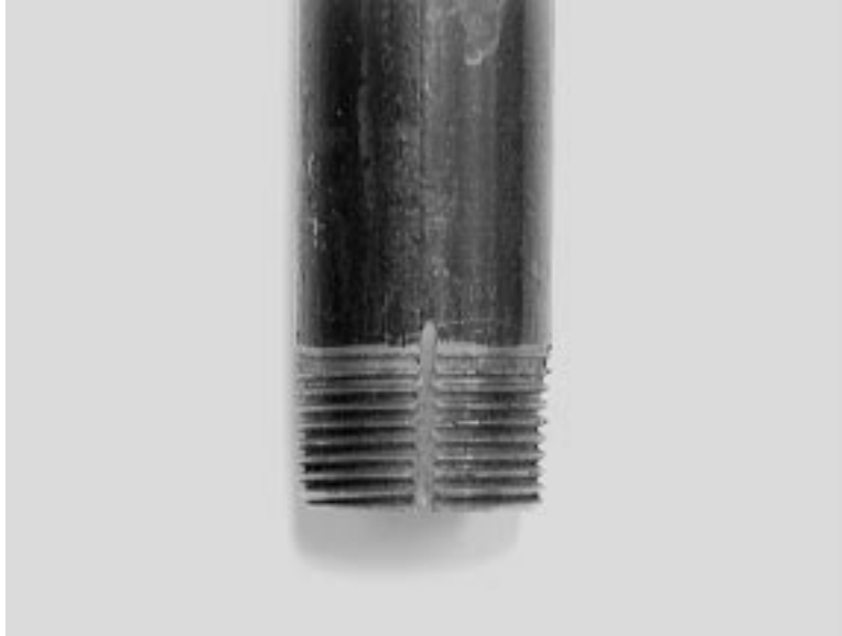
Figure 3-6 Groove Cut in Threads to Induce Water Leakage
