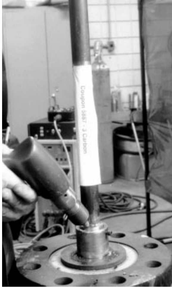
Figure 4-2 Mechanical Peening of Socket Weld
