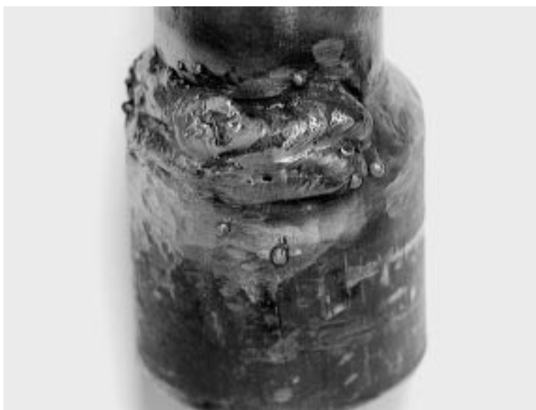
Figure 4-9 Test Coupon CST-2 after Welding
