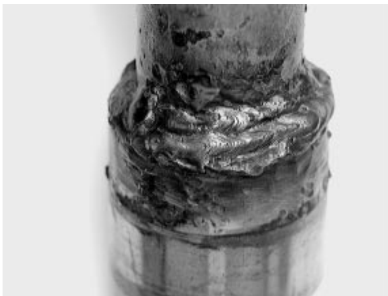
Figure 4-19 Test Coupon SST-1 after Welding
