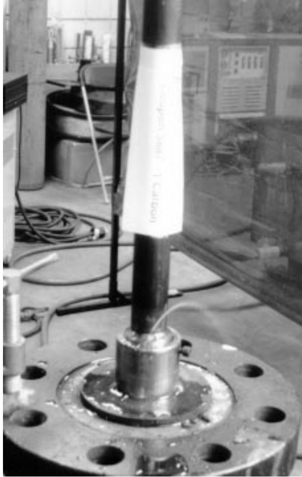
Figure 4-1 Water Leakage from Socket Weld Coupon under Pressure
