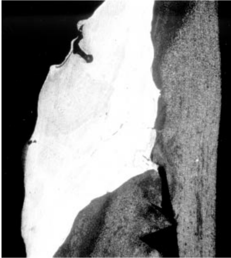
Figure 4-10 Cross-Section of Weld Repair on Coupon CST-2 (Magnified 6.3x)
