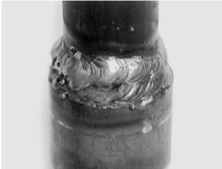
Figure 4-12 Test Coupon CST-3 after Welding
