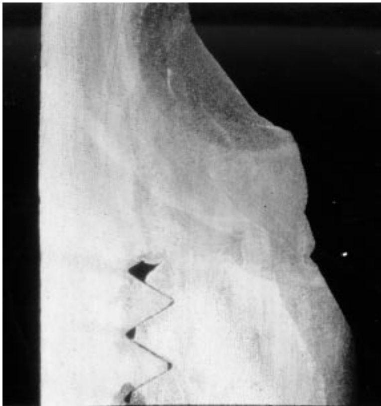
Figure 4-15 Cross-Section of Weld Repair on Coupon CST-5 (Magnified 6.3x)
