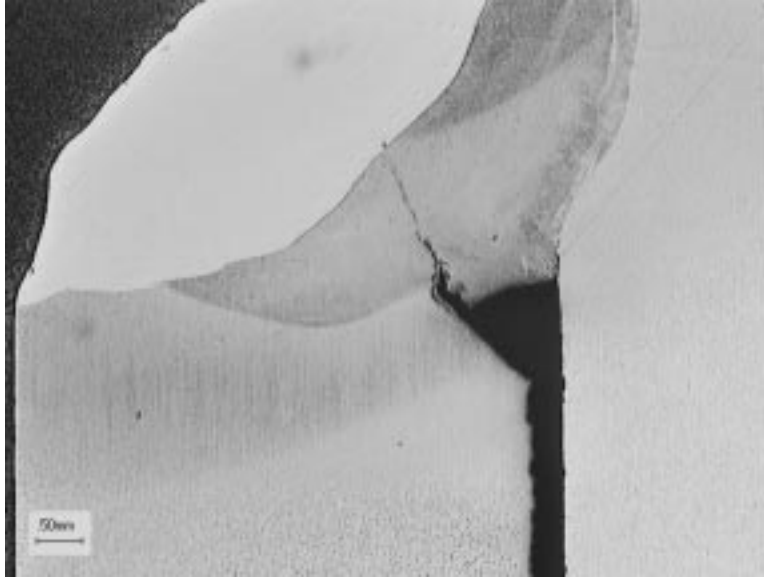
Figure 4-6 Cross-Section of Coupon CSS-2 Showing Fatigue Flaw Sealed by Welding (Magnified 10x)
