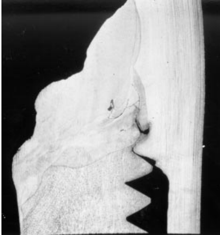
Figure 4-20 Cross-Section of Weld Repair on Coupon SST-1 (Magnified 6.3x)
