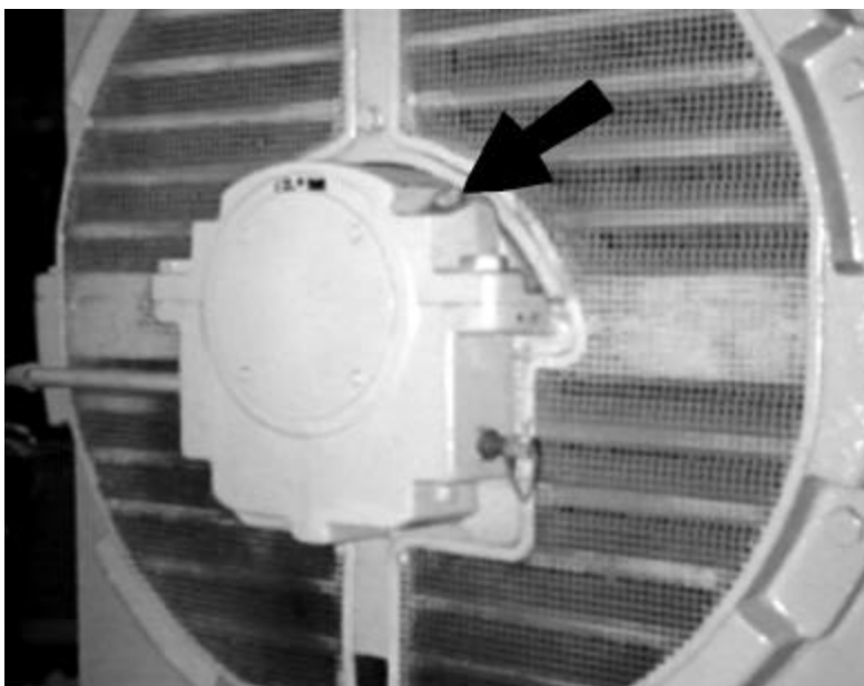
Figure 3-4 Sampling from Bearing Fill Plug - Ball Bearing, Outboard Motor
