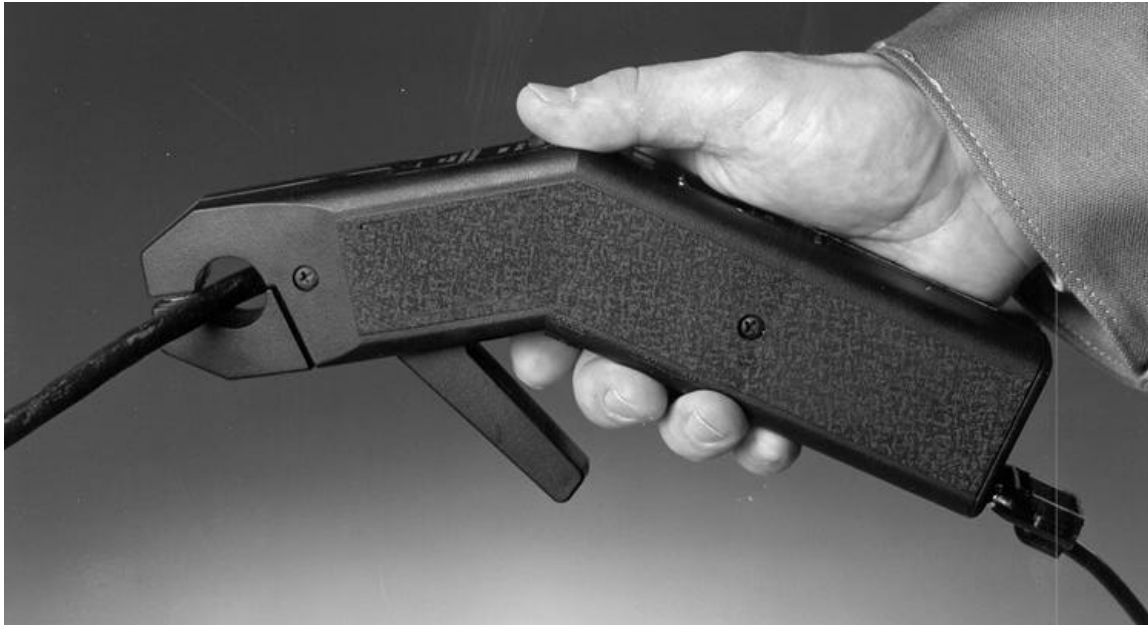
Figure 5-4 Current probe used for motor current monitoring
