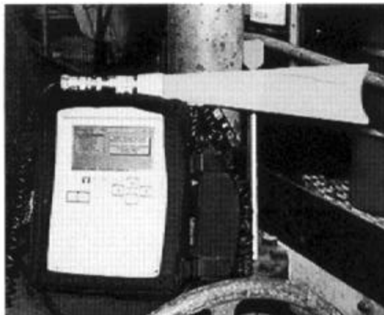
Figure 6-3 Data Collector with Shaft-Stick Attachment
