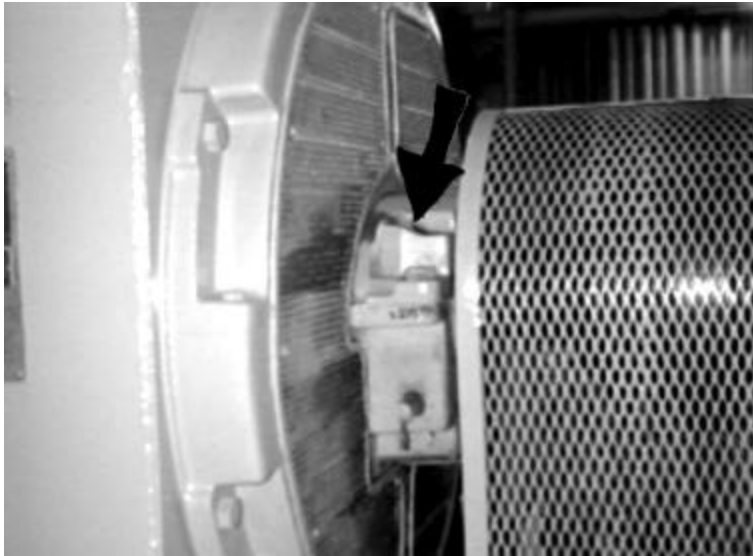
Figure 3-5 Sampling from Bearing Fill Plug - Ball Bearing, Inboard
