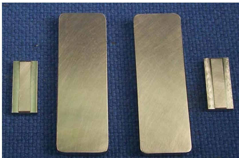
Figure 3-4 Lapped Flat-on-Flat Autoclave Test Samples. The larger samples are the moving inner samples (1" x 3")
