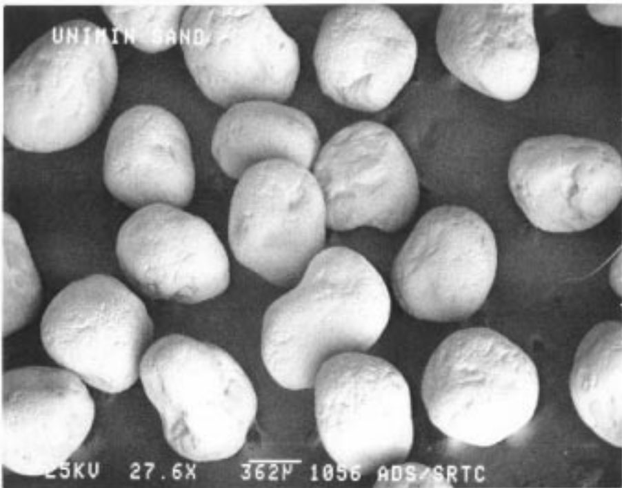
Figure 2-1 Scanning electron micrographs of the crushed tuff (top) and quartz (bottom) used as matrix material in this study. The quartz was slightly larger and appreciably smoother than the crushed tuff.
