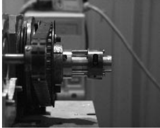
Figure 3-30 Welding Set-Up for Powder Welded Insert Configurations
