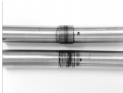
Figure 3-21 Internal Weld Trials On Tube #5 (Top) And #6 (Bottom)
