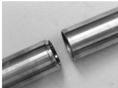
Figure 3-28 Final Step in Laser Powder Insert Build Up
