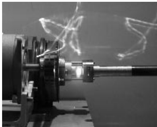
Figure 3-31 Inserting the Weld Head into the Tube-to-Tube Connection
