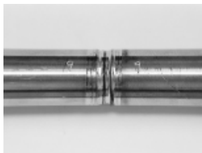
Figure 3-11 Externally Delivered Beam Weld Tests—Weld #9
