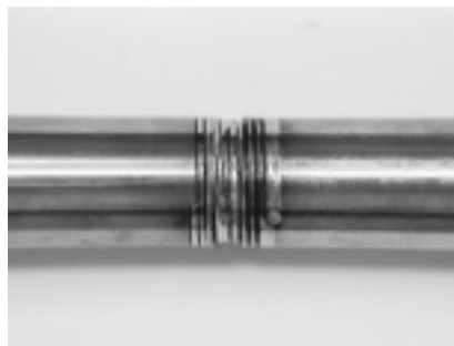
Figure 3-13 Externally Delivered Beam Weld Tests—Weld #11
