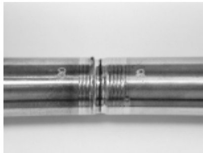
Figure 3-10 Externally Delivered Beam Weld Tests—Weld #8
