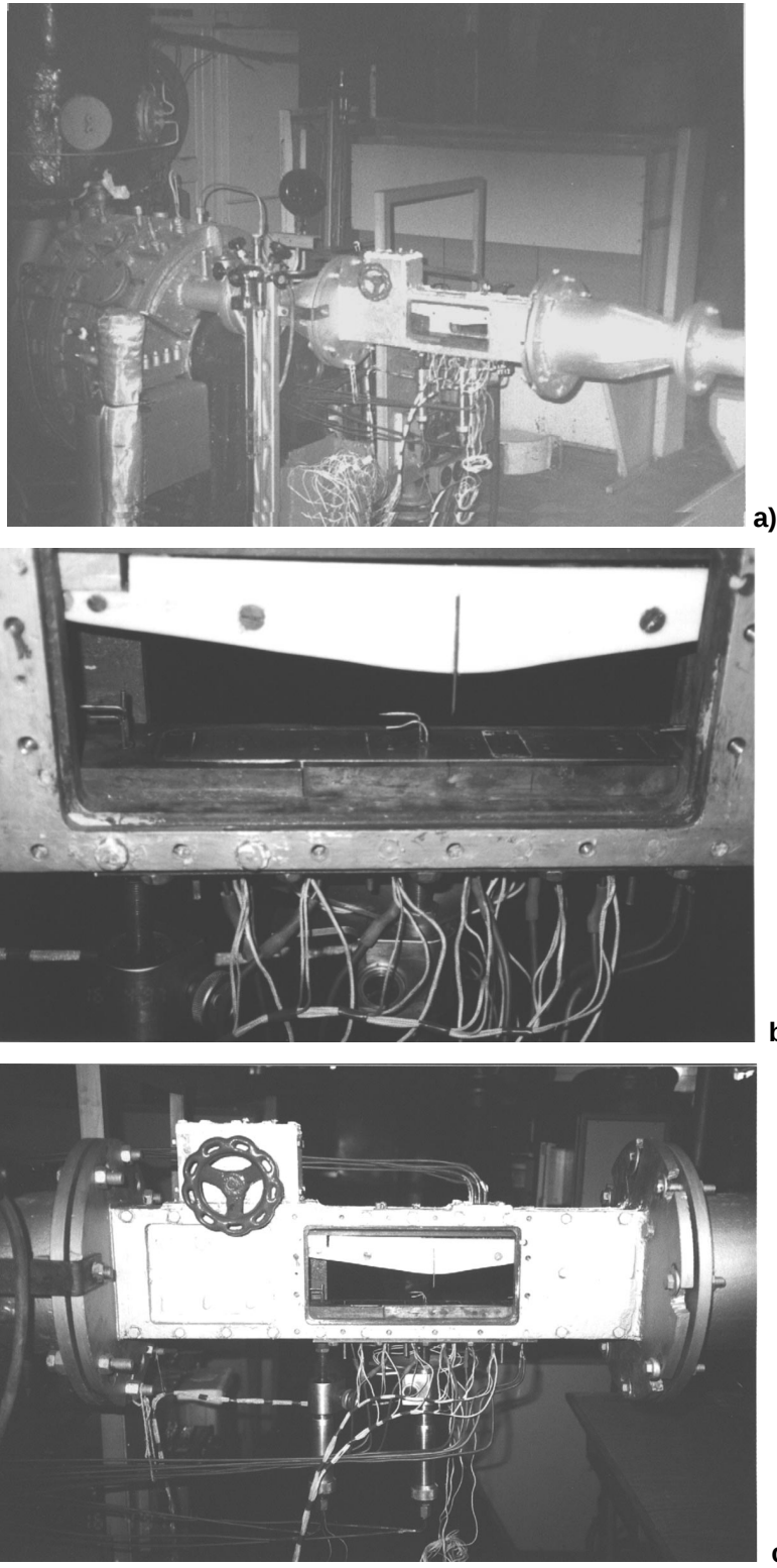
Figure 2-4 The Wet-Steam Rig with the Test Turbine Installed Upstream (a); the Working Part of the Rig (b); the Test Channel with the Movable Upper Profile (c)
