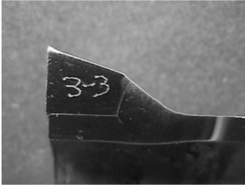
Figure 4-1 Root Failure (3/4" (1.91 cm) 2 x 1 Weld)
