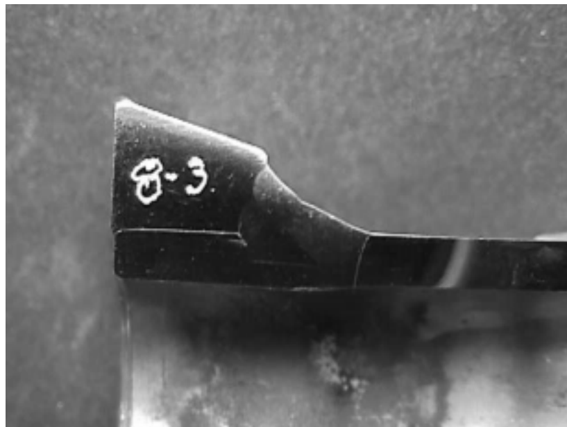
Figure 4-2 Toe Failure (3/4" (1.91 cm) Last Pass Improved)
