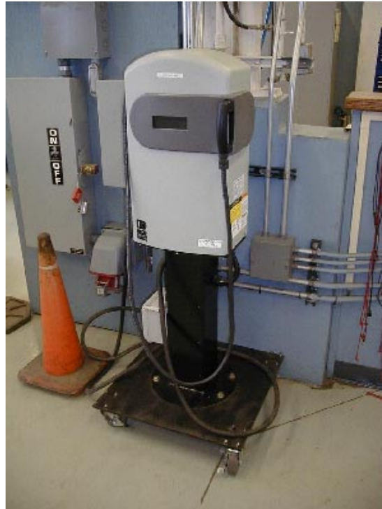
Figure 3-2 Hughes 6.6 kW Gen II Inductive Charger
