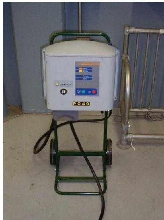
Figure 3-3 Toyota RAV4 Off-board Conductive EVSE, with Yazaki Connector (charger on-board)
