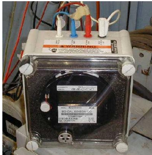
Figure 2-4 Portable ABB FM2S Watt-hour Meter
