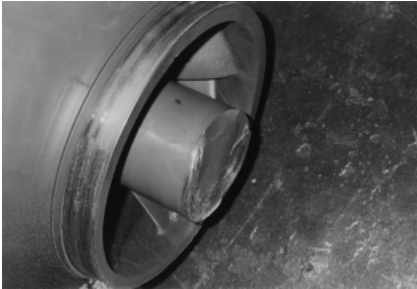
Figure 12-7 Heat Spots From Straightening 34APKD Shaft
