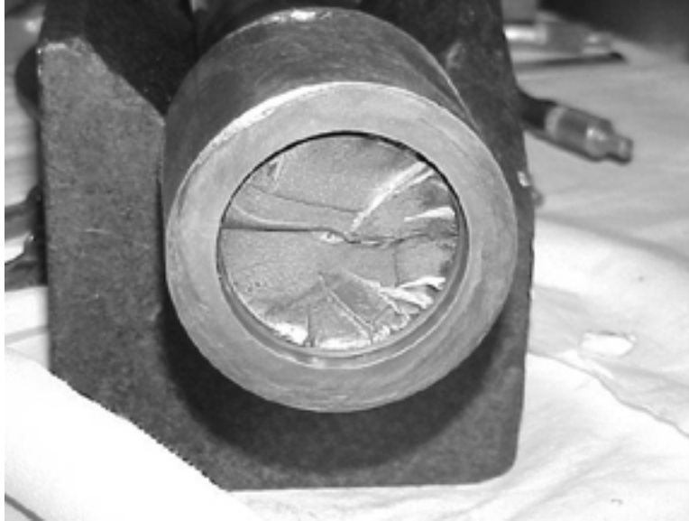
Figure 12-1 High Cycle Fatigue Failure of a Pump Shaft
