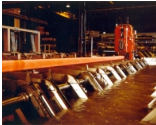
Figure 3-2 Direct Resistance Heating of Automotive Stabilizer Bars for Upsetting and Annealing
