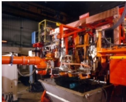
Figure 3-3 Direct Resistance Heating of 26' long x 5" Diameter Steel Bar to 1000°C in 13 Minutes
